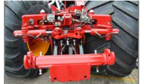
Hitch with active suspension and auto-controlled in crab steering
