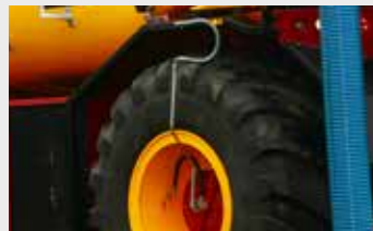
Tyre pressure control system for optimum tyre pressure on the road and in the field
