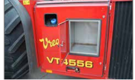
Water tank for washing hands, etc. and a handy storage box for PPE.
