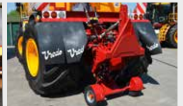
Extra assist Axle to meet Public safety and local regulations in case of loading additional heavy equipment.
