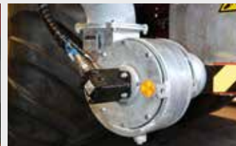
Turbo filler for increased loading capacity
