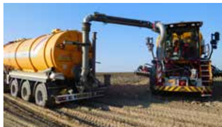
A 135° rotatable and telescopic reload arm gives great docking flexibility
