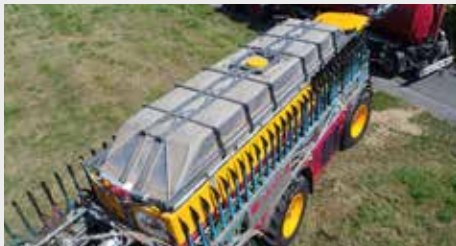
7m3 pumpable liquid bag on top of 25m3 polyester tank. (FlexTank)
