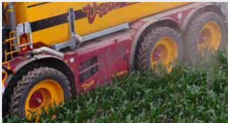
Row-crop wheels for driving in between the corn rows
