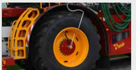
Tyre pressure control system for optimum tyre pressure on the road and in the field
