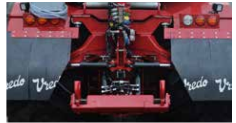
Hitch with active implement suspension and auto-controlled in crab steering
