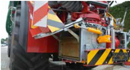
Slicing filter with automatic ejection function, operated from the cab
