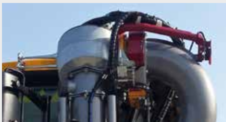
Centrifugal pump for very short reload time, up to 16.000 liters/min
