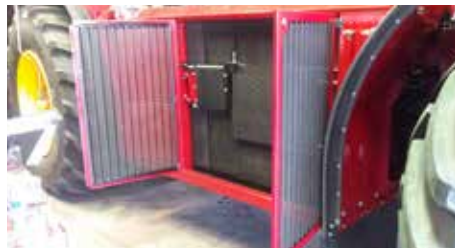
Cooling system with reversible fan, easy to clean - maximum cooling capacity
