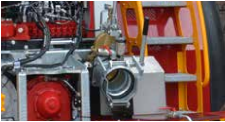
6" female reload connector. At opening the pump starts automatically
