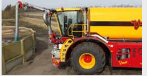
Extra long silo reload arm with centrifugal pump (Superload)
