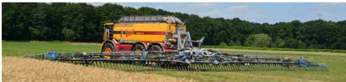
Up to 30 meter sliding-shoe applicator
