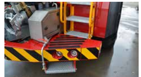
Clean water tank for washing hands, and a handy storage box for PPE
