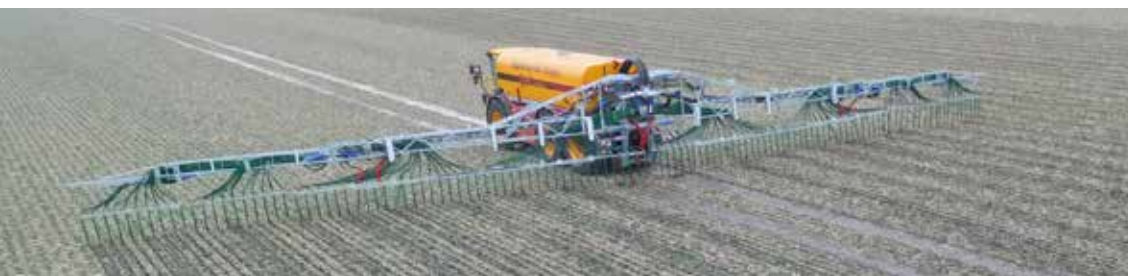
Up to 36 meter dribble-bar applicator
